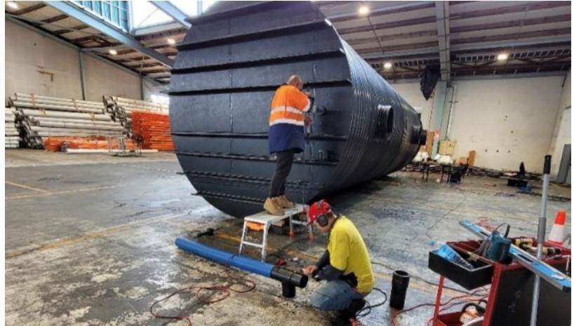
A fire tank (and its pipe fitting) being fabricated before its journey to the Waikato
