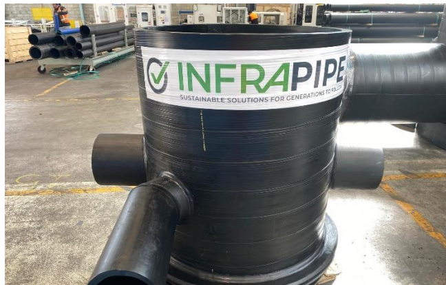
Fig 7. Manhole showing proximity of connections
