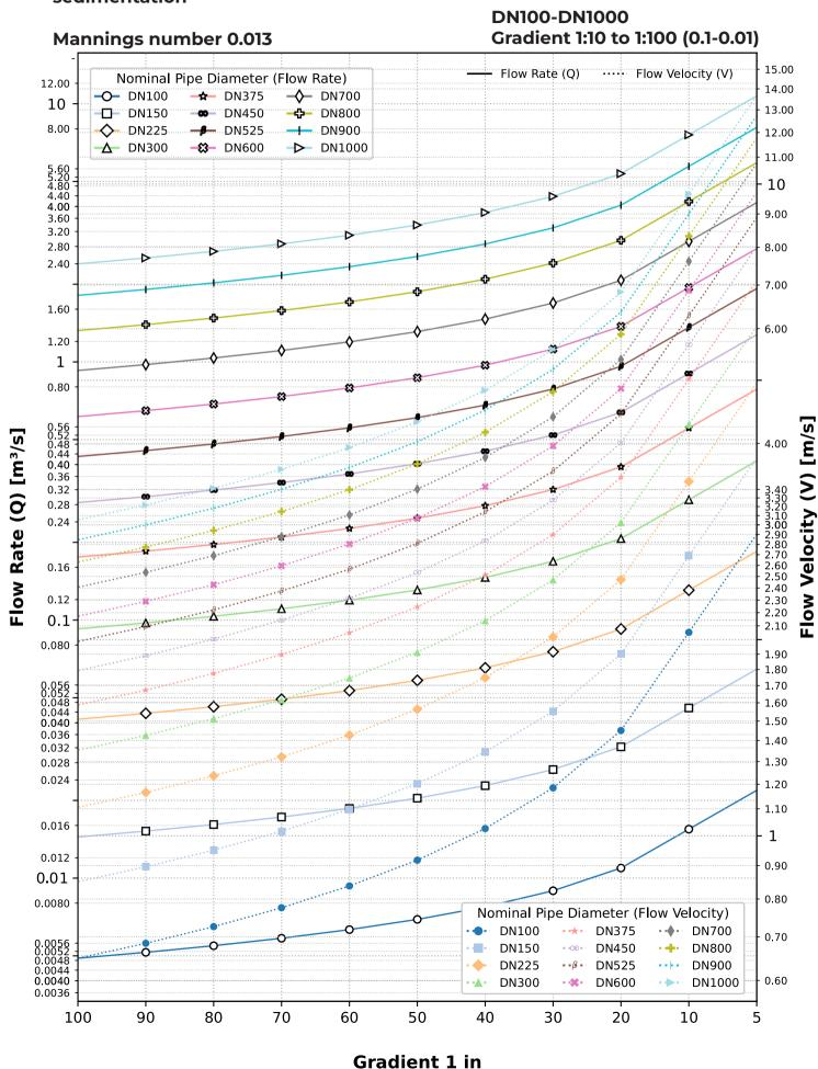
For HDPE/PP pipes with wear and sedimentation
