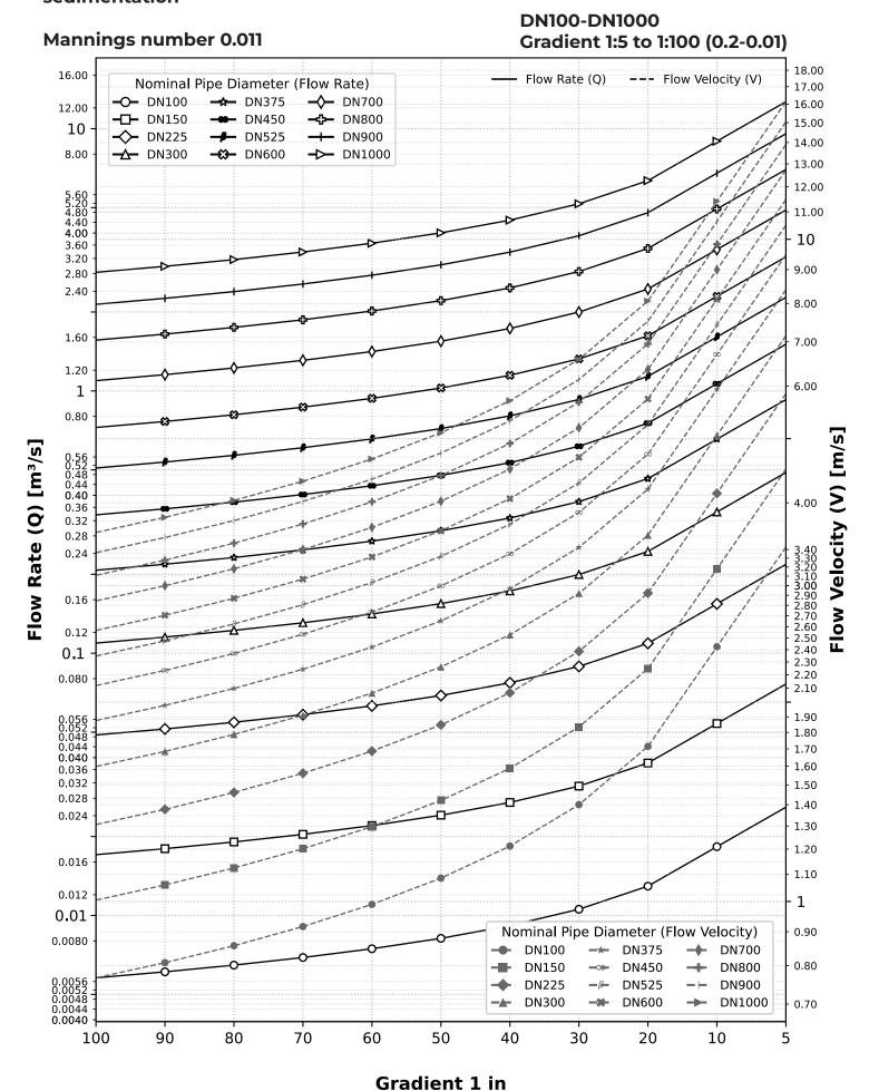
For HDPE/PP pipes with low wear or sedimentation
