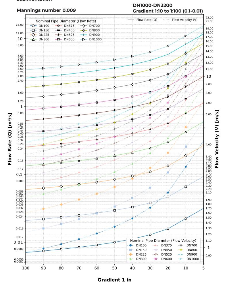
For HDPE/PP pipes with very low or nil sedimentation
