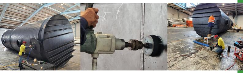
The tank's design can have **multiple fittings** added due to the requirements needed for water entering and leaving the tank.
